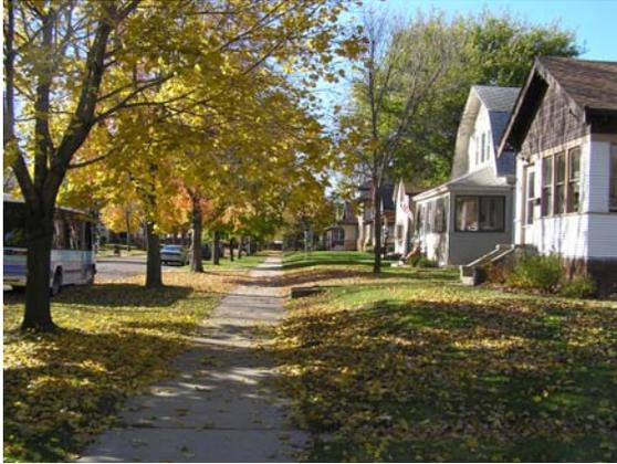
The curb system is a barrier curb. Although more costly to install, this system adds definition to the home site. The limited front yard makes the area feel safer and provides better security for the pedestrian and for the home owner. The boulevard planted with deciduous trees creates a psychological barrier between the street and the pedestrian on the sidewalk.
